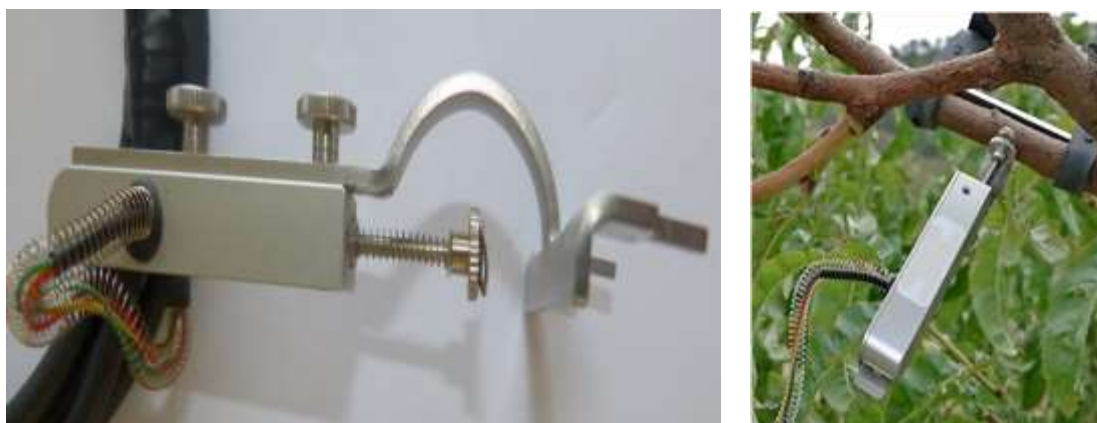
Figure 1. Dendrometer off and in situ
