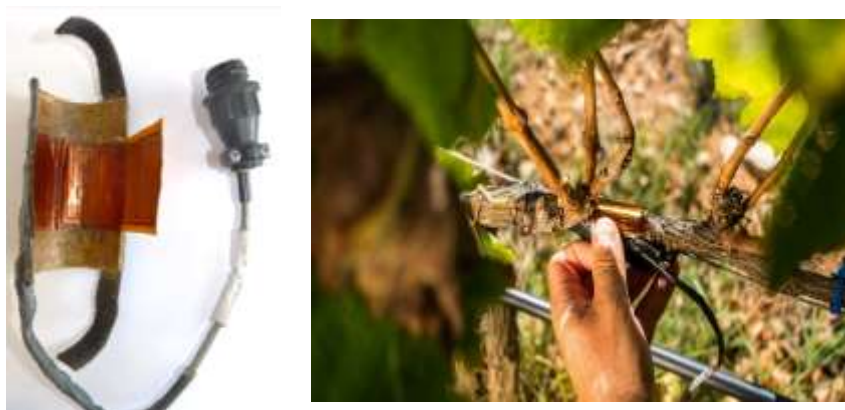
Figure 2. Sap flow sensor, off and in situ
